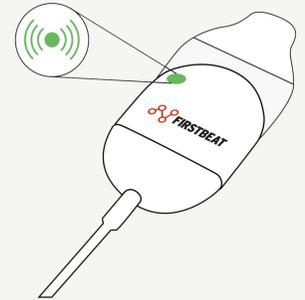
4. The measurement starts and green LED starts blinking when the device is attached to body and measurement is started from app. Note: The light is easiest to see in a dark room.
