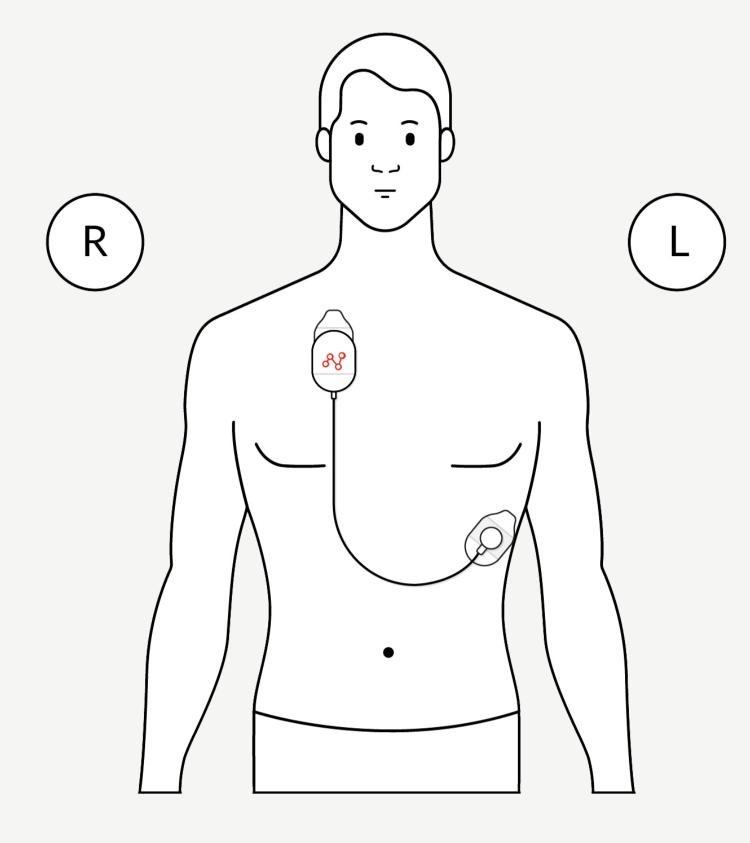
3. Attach the recorder to the right side of the body under the collarbone and the electrode cable end to the left side of the body on the rib cage.
