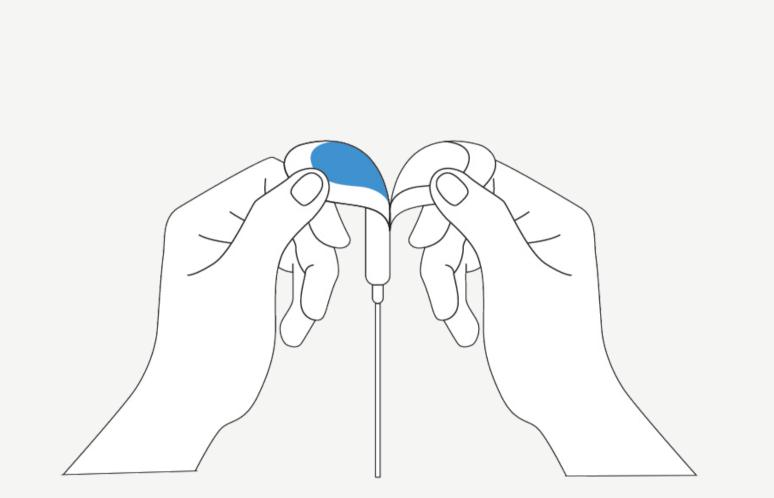
2. Remove the cover of the electrodes.
