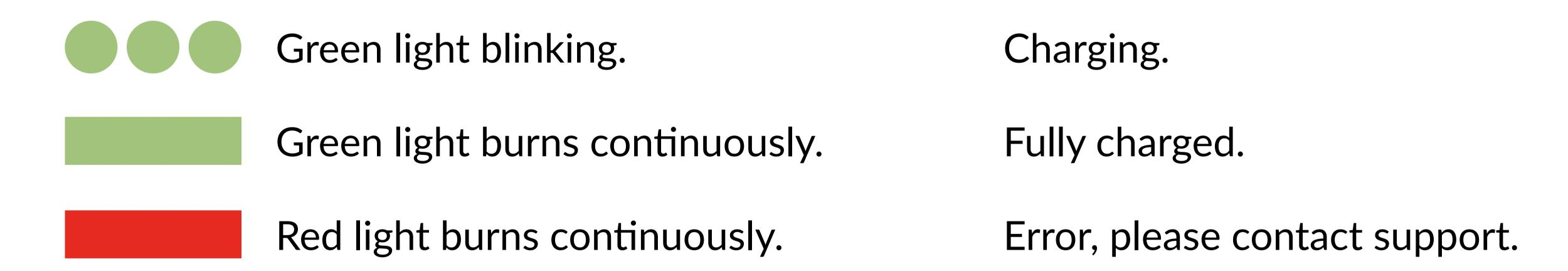
Note! To ensure the product is functioning to its full potential and to avoid damage to the battery the device must be charged at least once every four (4) months.
