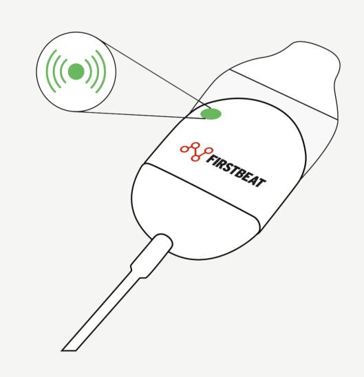
4. The measurement starts and green LED starts blinking when the device is attached to body and measurement is started from app. Note: The light is easiest to see in a dark room.
