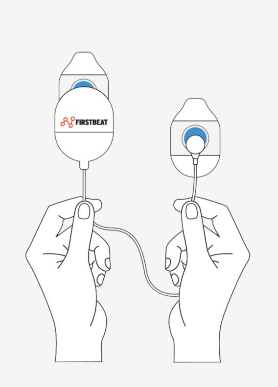
1. Attach electrodes to the recorder (the larger end of the device) and to the small circular end of the electrode cable.
